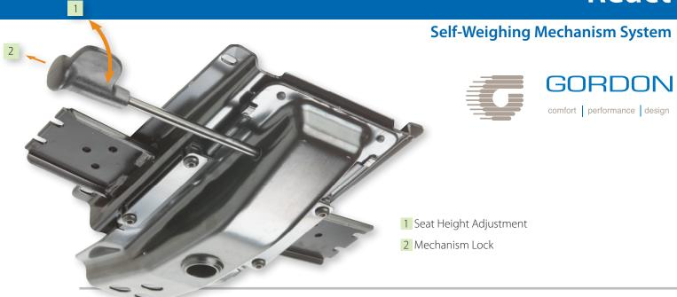
A breakthrough Self-Weighing Mechanism System, intuitively responds to torque requirements covering a wide range of users without the need for manual tension adjustment. The patented linked-motion configuration drives the reclining action by mechanically connecting the seat and chair back through an ergonomically positioned hip pivot design.
