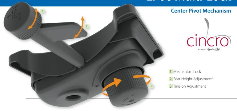
Center pivot mechanism for use with small to medium fixed back tilting chairs. This mechanism features a bottom knob for tension adjust and dual-function, combination rotational lever for its 5 position tilt lock and chair height adjustment.
