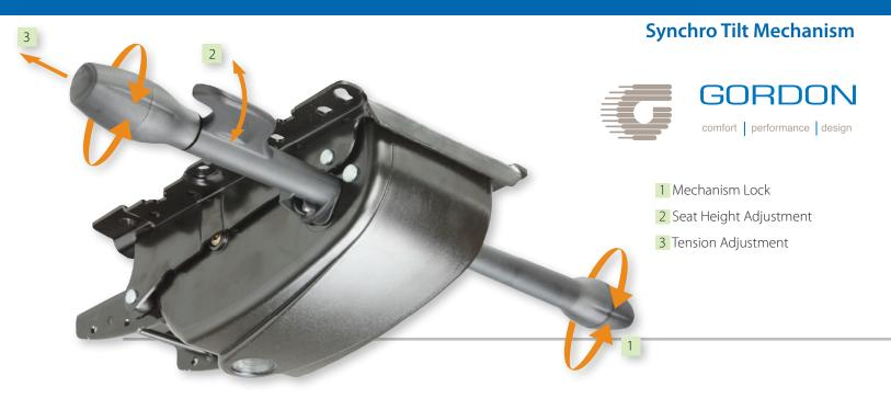
Forward pivot synchro mechanism with side tension adjustment. Engineered to provide proper tension and adjustability while maintaining even support throughout the entire travel range. 5 position tilt lock feature is designed with an anti-kickback safety feature.
